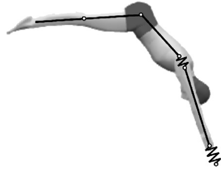
Fig. 2. The four-segment gymnast-high bar simulation model with damped springs representing bar and shoulder elasticity.
