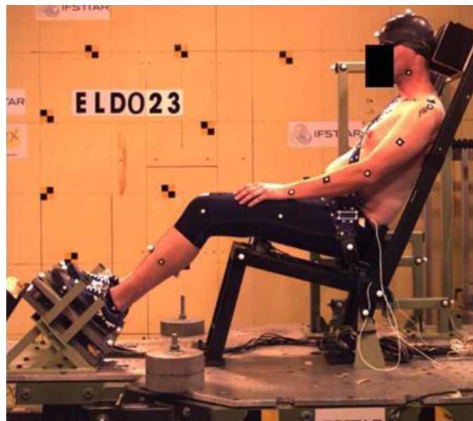
Fig. 1. Sled configuration based upon a standard sedan car environment of a front passenger restrained by a 3-point belt.
