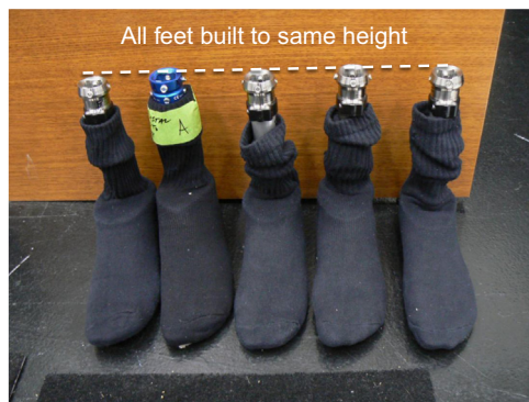
Fig. 1. Each prosthetic foot tested was built to the same height to facilitate quick swapping during laboratory kinetic testing. Feet were covered with black socks zip-tied to the pylon to obscure the foot make and model from the investigators, the participants and the statistician.
