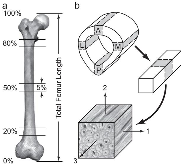
**Fig. 1.** Cortical bone specimens were sectioned from the diaphysis of whole human femora at (a) 20%, 50%, and 80% of the total femur length and (b) from each anatomic quadrant (A=anterior, M=medial, P=posterior, L=lateral), using an orthogonal curvilinear coordinate system (1=radial, 2=circumferential, 3=longitudinal).
