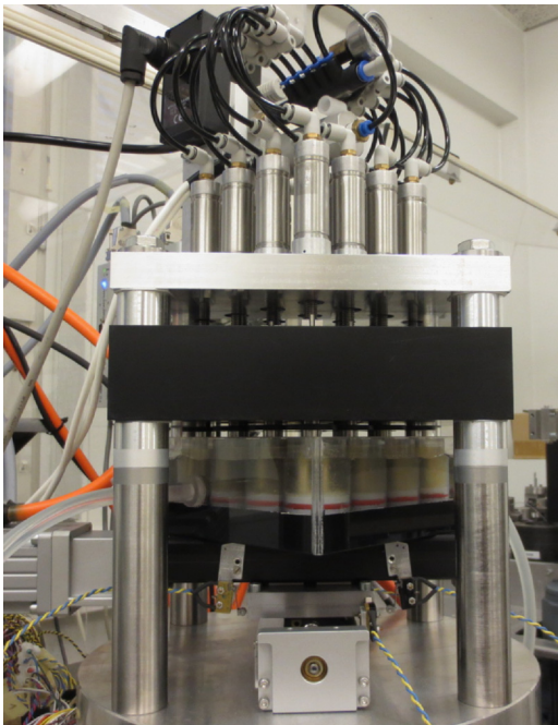
Fig. 1. Ball-on-flat test ongoing in 16-station RandomPOD. Note servo-electric x - y -stage and circulating cooling water surrounding test chambers that contain serum lubricant. Size of motion plate is 135 \text{ mm} \times 135 \text{ mm} . On top is proportional-pneumatic loading module.
