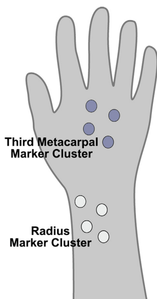
Fig. 1. Marker Placement. A cluster ( n = 4 , 6.4 mm dia.) of retroreflective markers placed on the dorsal side of the third metacarpal (MC3) and a cluster ( n = 4 , 6.4 mm dia.) of retroreflective markers placed on the dorsal side of the radius was used for optical motion capture (OMC) data collection.
