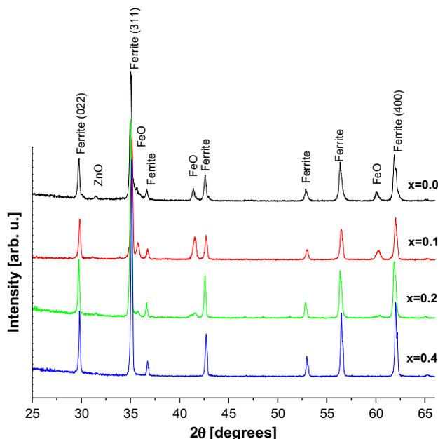
**Fig. 1.** X-ray diffraction patterns of samples  $\text{Li}_{0.5x}\text{Zn}_{0.6-x}\text{Mn}_{0.4}\text{Fe}_{2+0.5x}\text{O}_4$  ( $x = 0.0; 0.1; 0.2; 0.4$ ).
