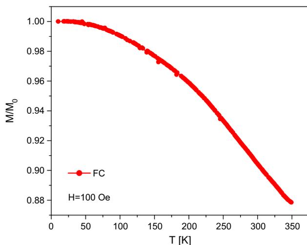
**Fig. 5.** Field cooling  $M(T)$  curve for sample 800. The applied field is  $H = 100$  Oe.
