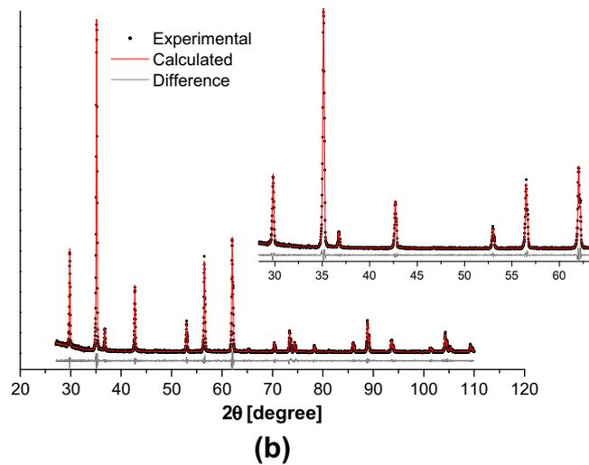
**Fig. 3.** Rietveld refinement of samples 801 (a, grey online) and 804 (b, red online). The inset is an enlargement of the portion with the most intense peaks. Circles indicate the observed intensity while the calculated pattern is shown as a solid curve. Below each spectrum, the difference between observed and calculated intensities can be seen. (For interpretation of the references to colour in this figure legend, the reader is referred to the web version of this article.)
