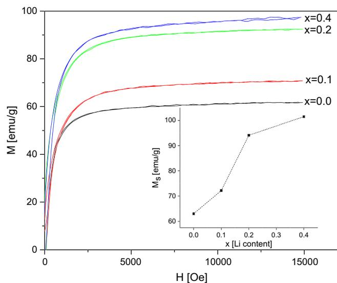
**Fig. 2.** First quadrant of the hysteresis loops for all the samples as a function of Li content,  $x$ . The inset shows the increasing of saturation magnetization with  $x$ , before correction for secondary phases.
