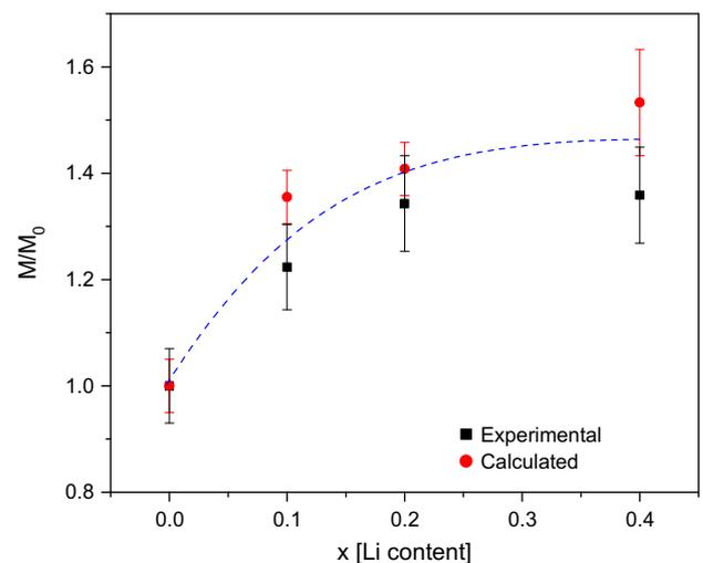
**Fig. 6.** Comparison between relative  ${}^xM_s^c$  (circles) and  ${}^xM_s^t$  (squares). The dashed line is a guide for the eye.
