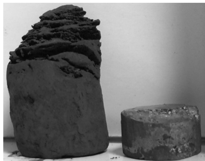
Fig. 8. Combustion products of Mo/Si/B/Ti mixture designed for 85% \text{Mo}_5\text{SiB}_2 and 15% \text{TiB}_2 . The left pellet was obtained by conventional SHS, while the right product was obtained by the chemical oven technique.
