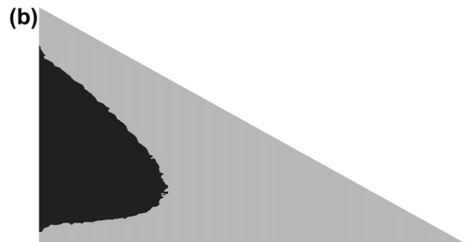
Fig. 12. Effect of cohesion c ( N_{el} = N_{cl} = 40 ). (a) vertical base pressure; (b) predicted plastic zone with c_{dp} = 1000 Pa.
