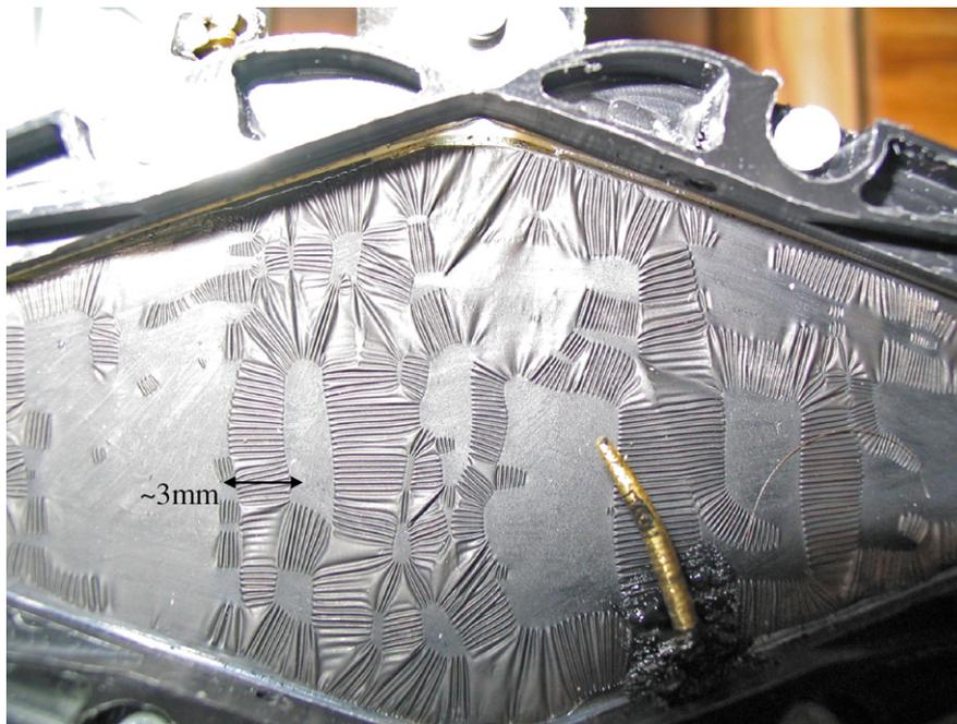
Fig. 1. An experimental observation of electromechanical instability (courtesy of Plante and Dubowsky). A layer of a dielectric elastomer, coated with conductive grease on top and bottom faces, is pre-stretched using a frame. An electric voltage is applied between the two electrodes. The layer deforms into a mixture of two regions, one being flat and the other wrinkled. For further experimental details see Plante and Dubowsky (2006).
