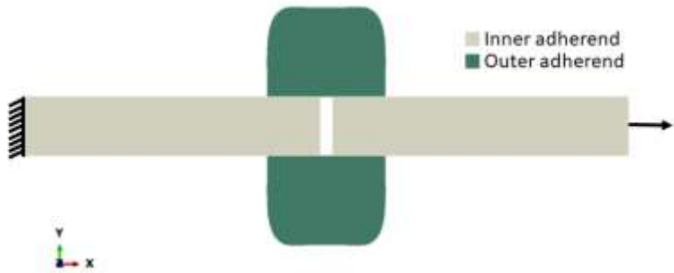
Figure 5 analysis setup for tensile loading condition
