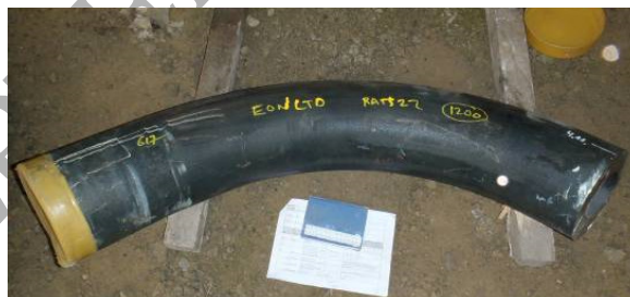
Figure 3: Section of Alloy 617 piping used for experimentation (shown alongside A4 sheet of paper as size comparison)
