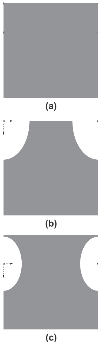
Fig. 12. Topology optimization through insertion of infinitesimal holes into structure of Fig. 11: (a) optimal hole locations identified, (b) optimal size of the two holes initially placed at the upper corners, and (c) optimal size of the two holes initially placed at the lower locations.
