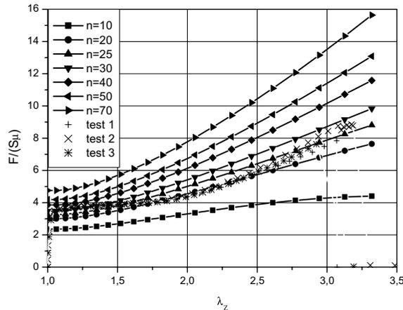
Fig. 15.  $T_Z - \lambda_Z$  curves according to the three-term Rivlin's model for different values of  $n$ .
