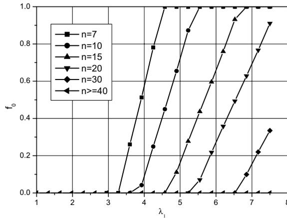
Fig. 2. Evolution of the porosity  $f_0$  for different  $n$  under uniaxial tension.
