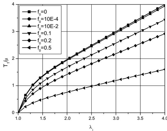
Fig. 3. Neo-Hookean laws for equi-biaxial tension with different fixed porosities  $f_0$ .
