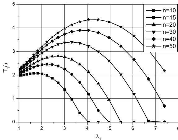
Fig. 6. Neo-Hookean laws for hydrostatic tension with growing porosity.
