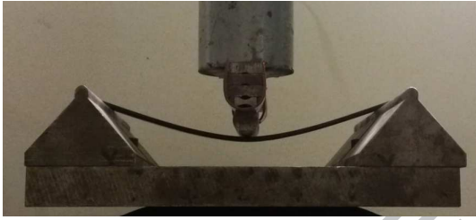
Figure 16: The experimental setup for the three-point bending test of an SMA beam.
