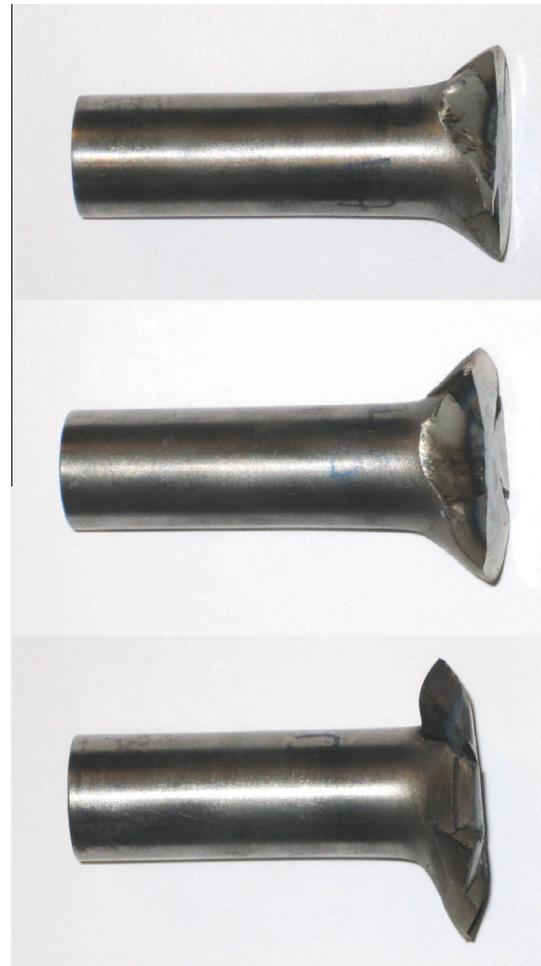
Fig. 14. HRC 40 projectiles after impact at velocities of 297.7, 325.6, and 356.6 m/s, respectively.
