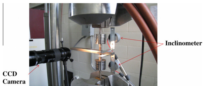
Fig. 6. DCB specimen attached with inclinometer during the peel test.
