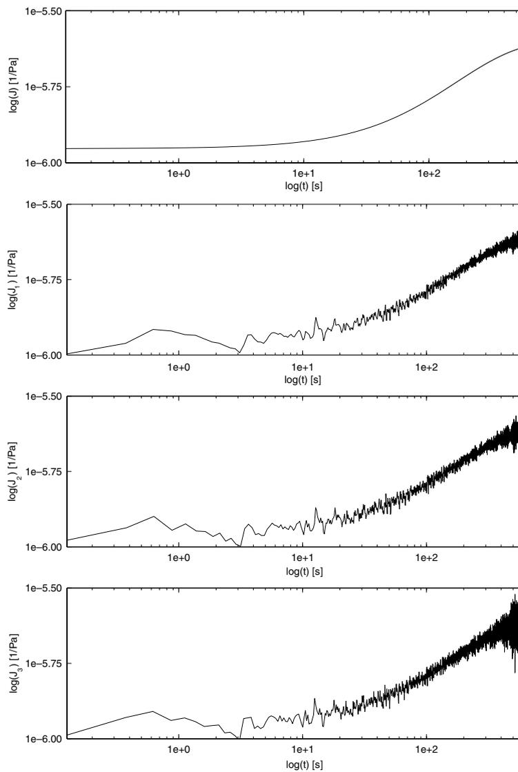
Fig. 5. Tikhonov regularized creep compliances for simulation case 6 with 20% noise. Figures from top to bottom correspond to analytical solution and Methods 1–3, respectively.
