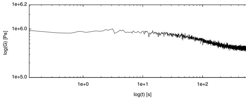
Fig. 4. Relaxation modulus as a function of time for simulation case 6 with 20% noise.
