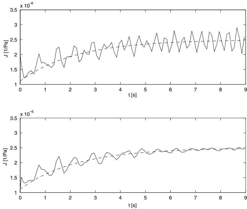
Fig. 3. Analytical (dashed line) and approximated (solid line) creep compliance without (upper figure) and with (lower figure) regularization for Method 1 in simulation case 7 with 10% noise.
