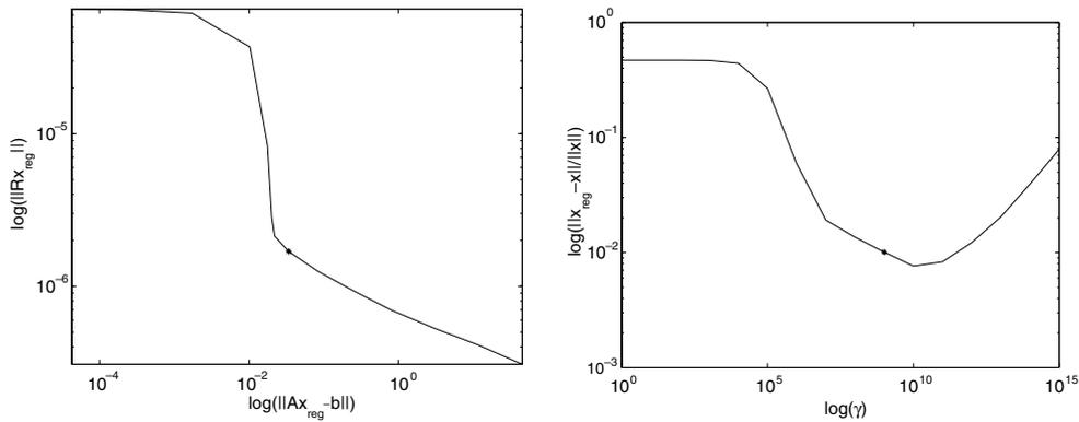
Fig. 2. Left: L-curve for Tikhonov regularization. Right: Real estimation error. The solution according to value  $\gamma = 10^9$  is shown with the star (\*) in both graphs.
