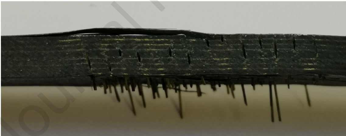
Figure 11. Upper half laminate of DCB test specimen after test showing buckling and delamination in the outer layers.
