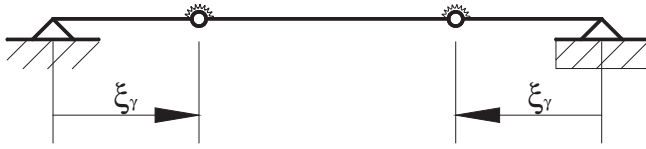
Fig. 4. A simply supported column with two cracks at symmetric cross-sections.
