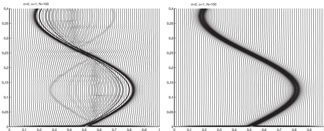
Fig. 2. Numerical results for the one-dimensional-advection model: an irregular adaptive grid for  $\sigma = 0$  (left) vs. a smooth adaptive grid for  $\sigma = 2$  (right).
