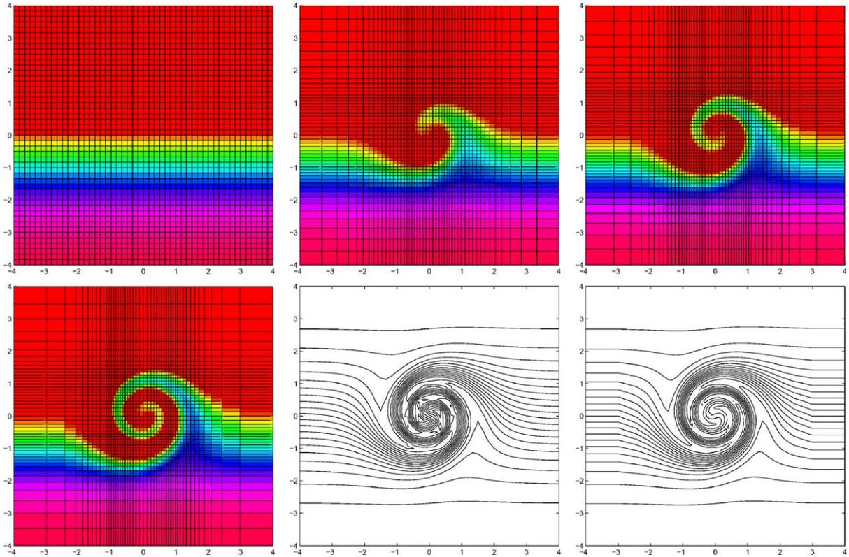
Fig. 3. Tensor-grid solutions for the whirlpool model at  $t = 0.0, 1.6, 2.8, 4.0$  and contourplots at  $t = 4$ : uniform grid vs. adaptive grid (right).
