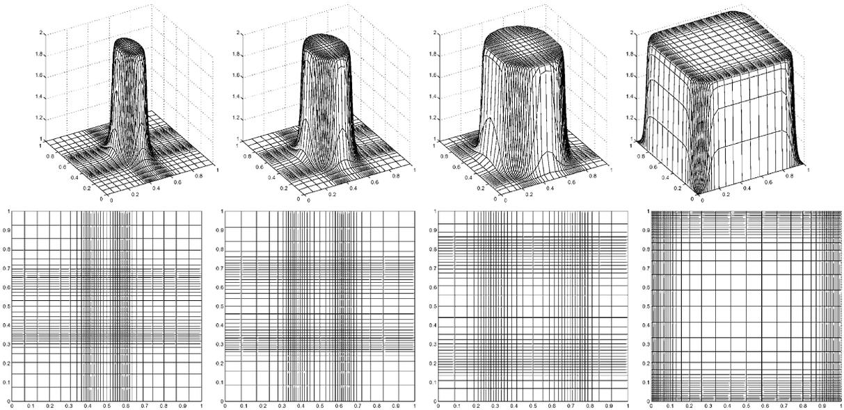
Fig. 4. Tensor-grid solutions for the combustion model at  $t = 0.01, 0.02, 0.04, 0.08$ .
