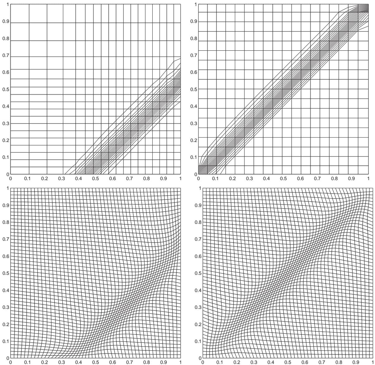
Fig. 6. Tensor-grids with exact contour lines of the solution (upper) compared with fully two-dimensional adaptive grids (lower) for the scalar two-dimensional Burgers' equation at  $t = 0.5$  and  $t = 2$ .
