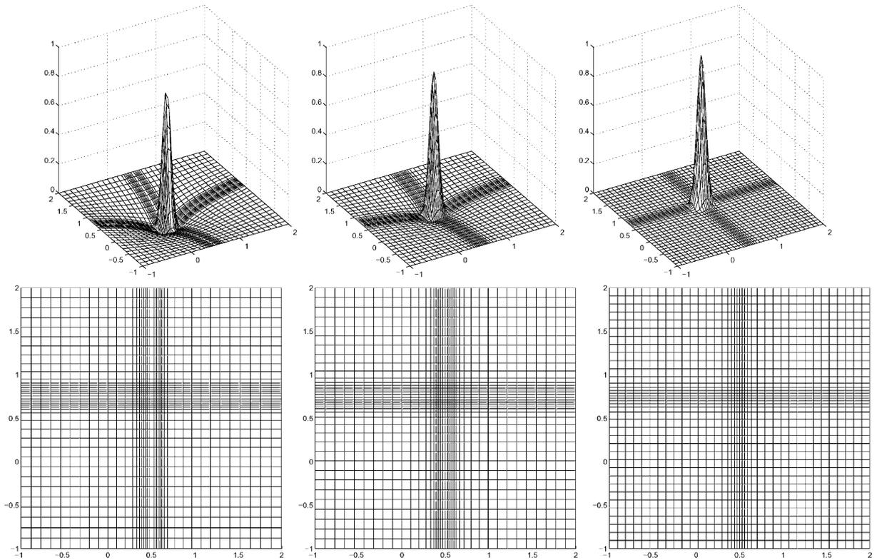
Fig. 7. Tensor-grid solutions for the rotating cone model: solutions and grids after one rotation for, respectively,  $(\alpha, \sigma) = (1, 0.2)$ ,  $(\alpha, \sigma) = (1, 1)$ , and  $(\tilde{\alpha}, \sigma) = (10, 0)$ .
