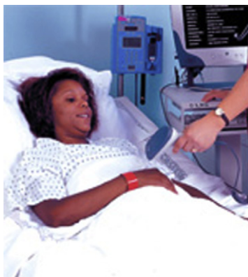
FIG E1. Handheld scanner attached to a screen and RFID-tagged wristband used at the Jacobi Medical Center in New York. Reproduced with permission from Siemens IT Services and Solutions. Available at: http://www.ti.com/rfid/docs/news/eNews/enewsvol40.htm . Accessed February 6, 2008.
