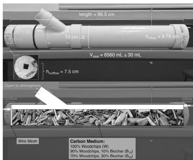
Fig. 1. Top: dimensions of horizontal flow bioreactor columns, where V_{\text{total}} is the total internal volume, and h_{\text{inflow}} and h_{\text{outflow}} are the heights of the inlet and outlet. Bottom: flow of simulated agricultural drainage is right to left and column headspace freely exchanges with the atmosphere through the wye. Note that volume of woodchips was the same for each treatment and the percentage of biochar is volumetric.
