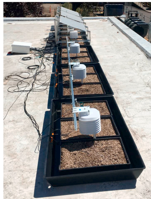
Fig. 1. Exposed (foreground) and shaded (background) experimental green roof modules (tubs) deployed on a rooftop in Corvallis, OR, USA.
