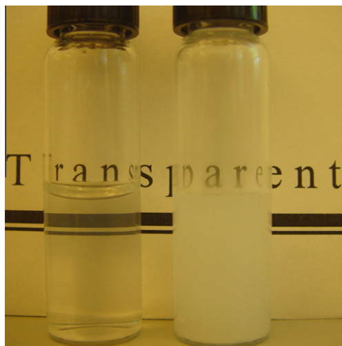
Fig. 1. POPC/POPS bilayers supported on \varnothing 20 nm (left) and \varnothing 100 nm (right) silica particles. Both samples contain the same interfacial area ( \sim 2 m 2 /sample) and the same amount of adsorbed lipids ( \sim 7 mg/sample) respectively.
