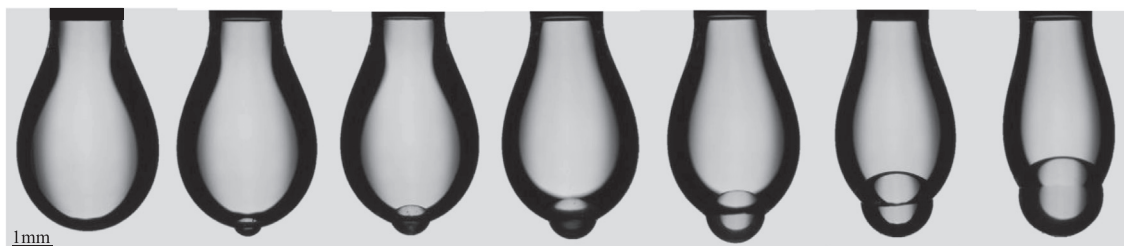
Fig. 4. Illustration of the drop loading with a glass bead at constant capillary force. The images correspond to pendant water drops just before their detachment and formed with a same needle of diameter ( D_{ne} = 1.80 mm) and an increasing load.
