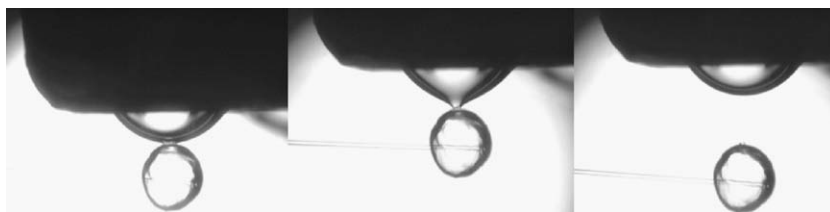
Fig. 7. When acids are present the water does not wet the hydrate as was seen in the systems without acids. The acids adsorbed to the hydrate surface reduce the water from bridging to the hydrate surface.
