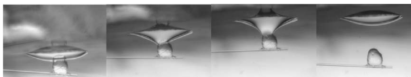
Fig. 5. General experimental image between hydrates and solid surfaces with a water drop deposited on the solid. The water is stretched until the hydrate particle detaches from the solid surface.
