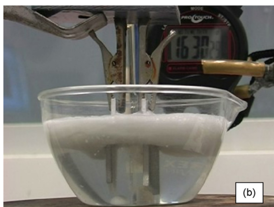
Fig. 3. Photographs during electrocoagulation of milk sample at 0.2 A in the presence of ammonium sulfate at 14'30" (a), 16'30" at rest (b).
