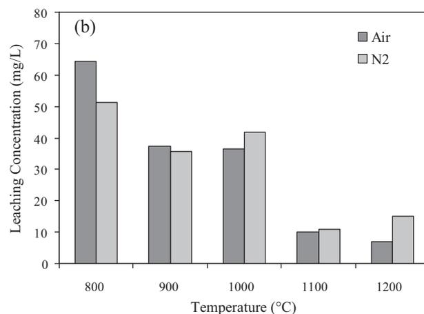
Fig. 10. Leaching concentrations of samples (with a Cr/Ni ratio of 2 and a conductivity of 0.2 ms/cm) sintered at different temperatures under two atmospheres.
