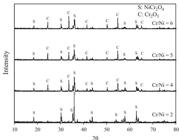
Fig. 7. XRD patterns of samples (with a conductivity of 3 ms/cm) with different molar ratios sintered at 1200 °C.
