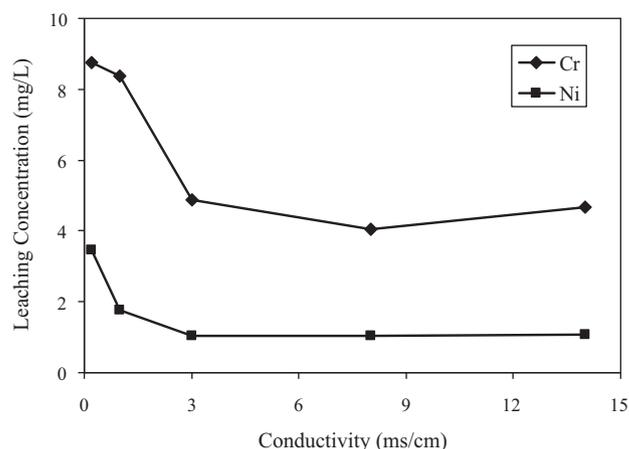
Fig. 6. Leaching concentrations of samples (with a Cr/Ni ratio of 2) with different conductivities sintered at  $1200^\circ\text{C}$ .
