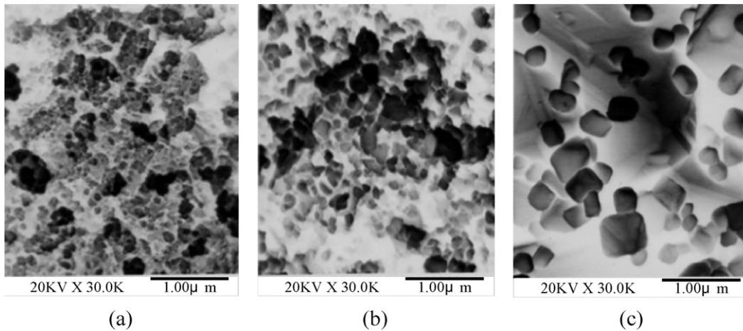
Fig. 2. SEM micrographs of samples (with a Cr/Ni ratio of 2 and a conductivity of 1.4 ms/cm) sintered at (a) 500, (b) 800, and (c) 1200 °C.
