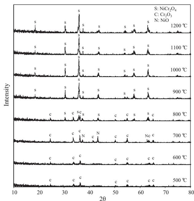
Fig. 1. XRD patterns of samples (with a Cr/Ni ratio of 2 and a conductivity of 1.4 ms/cm) sintered at different temperatures.
