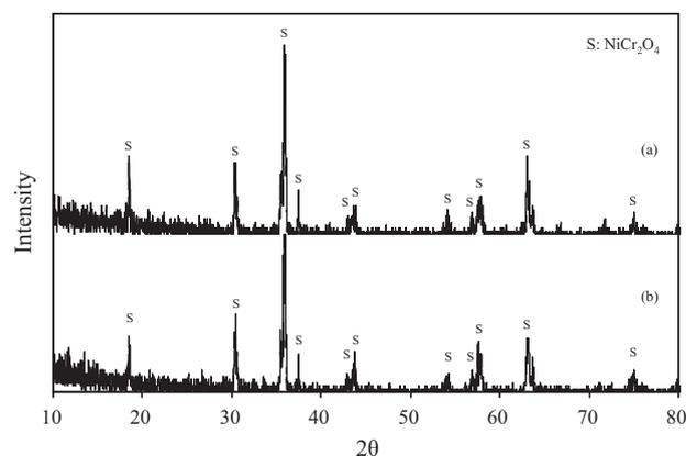
Fig. 9. XRD patterns of samples (with a Cr/Ni ratio of 2 and a conductivity of 0.2 ms/cm) sintered at 1200 °C under two atmospheres of (a) N<sub>2</sub> and (b) air.
