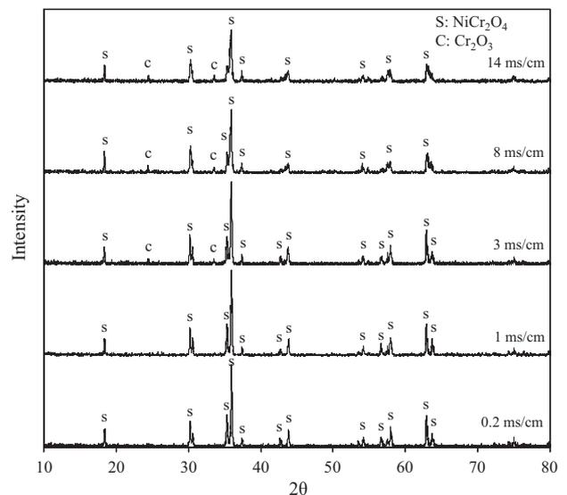
Fig. 4. XRD patterns of samples (with a Cr/Ni ratio of 2) with different conductivities sintered at 1200 °C.
