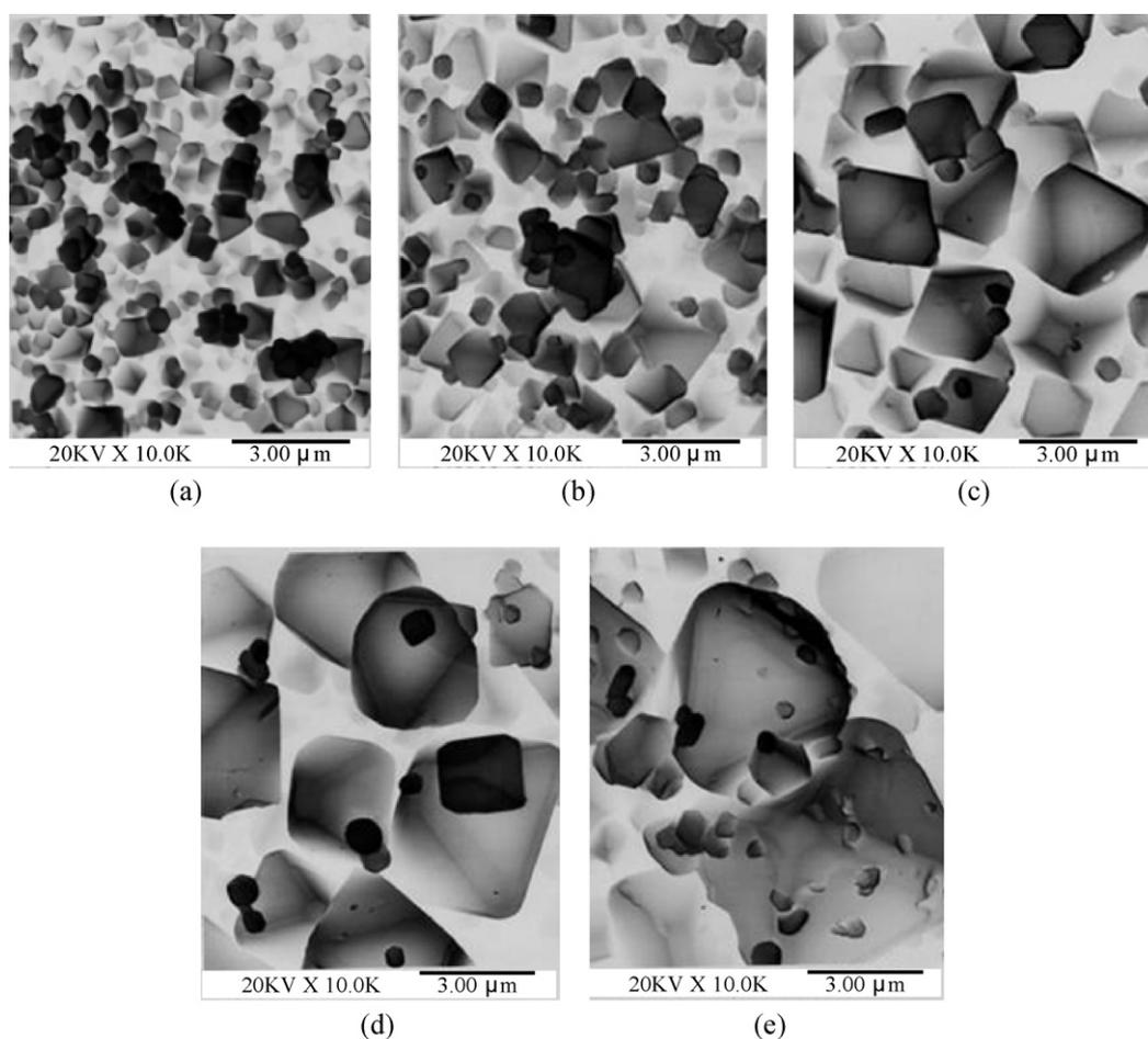
Fig. 5. SEM micrographs of samples (with a Cr/Ni ratio of 2) with different conductivities of (a) 0.2, (b) 1, (c) 3, (d) 8, and (e) 14 ms/cm.
