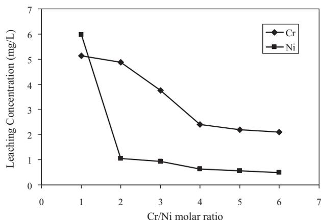
Fig. 8. Leaching concentrations of samples (with a conductivity of 3 ms/cm) with different molar ratios sintered at 1200 °C.
