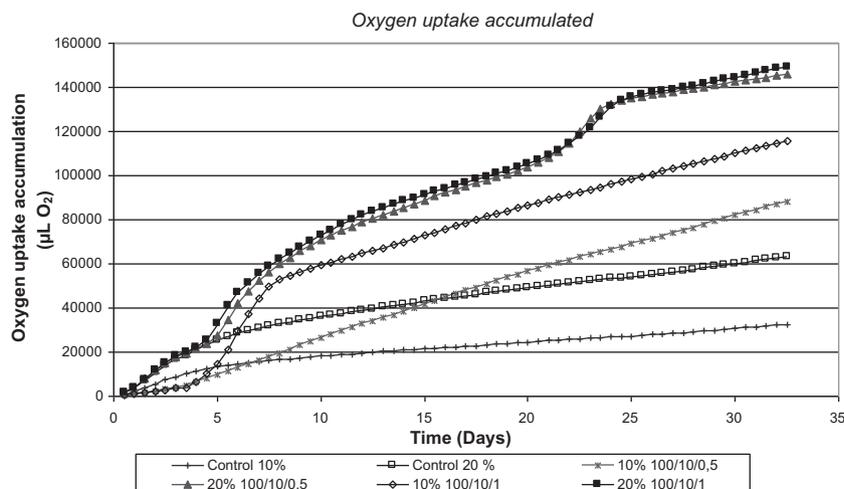
Fig. 1. Oxygen uptake evolution in tests performed at 10 and 20% pulp densities with different nutrient amendments.
