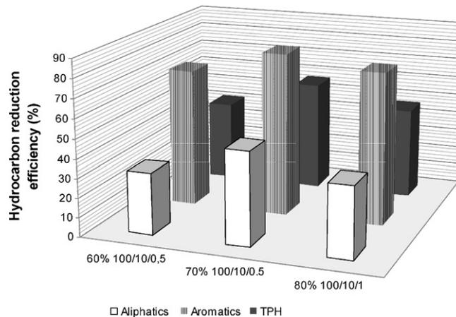
**Fig. 3.** Comparison of TPH reductions and total aromatic and aliphatic hydrocarbons at optimal conditions depending on humidity as a percentage of WHC.
