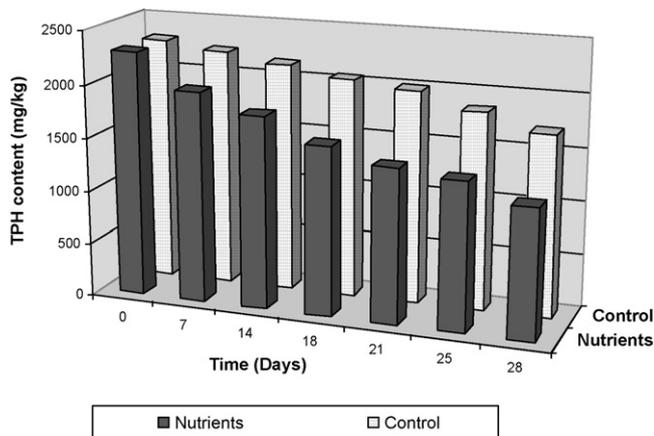
**Fig. 2.** The evolution of TPH content in tests performed at 20% pulp density in 2L reactors.
