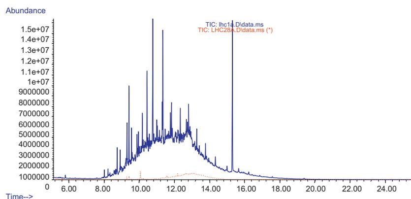
Fig. 7. Total ion chromatograms (GC/MS) of initial sample and optimal final samples (dotted line) obtained in mesocosms landfarming tests.
