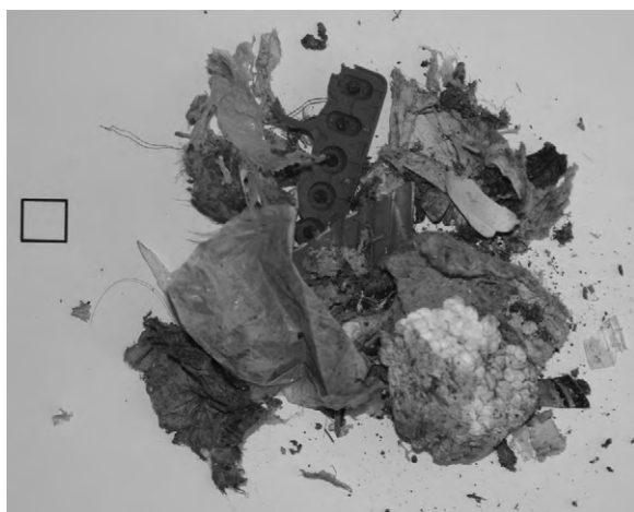
Fig. 2. Photograph of the incinerated RDF (the black square is 10 \times 10\text{ mm} ).
