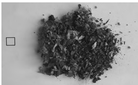
Fig. 3. Photograph of the incinerated ASR (the black square is 10 \times 10\text{ mm} ).
