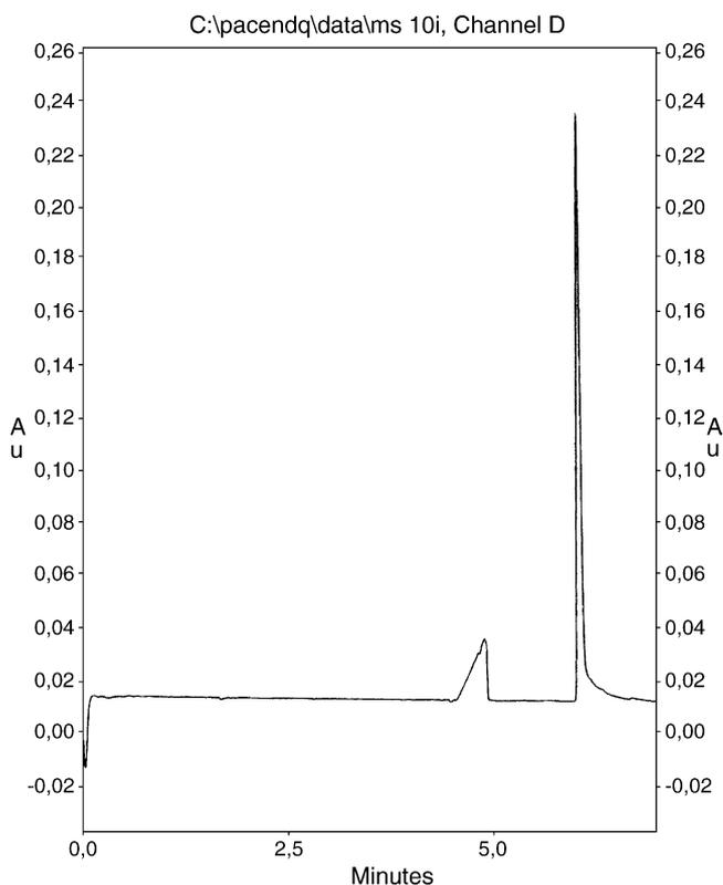
Fig. 1. Electropherogram of human saliva sample spiked with Pb(II). Conditions: 20 mM imidazole buffer containing 15% acetonitrile, pH 6.00; capillary, 57 cm full length, 50 cm effective length, 75  $\mu\text{m}$  i.d., 375  $\mu\text{m}$  o.d.; hydrodynamic injection at 0.5 psi, 5 s; 25 kV constant voltage; indirect UV detection at 205 nm.
