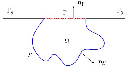
**Fig. 1.** The problem geometry. An open cavity with the wall  $S$  is placed on a perfectly conducting ground plane  $\Gamma_g$ . The aperture  $\Gamma$  covers the cavity and divides the physical domain into the interior  $\Omega$ , enclosed by  $S$  and  $\Gamma$ , and the upper half-space above the flat surface  $\Gamma_g \cup \Gamma$ .
