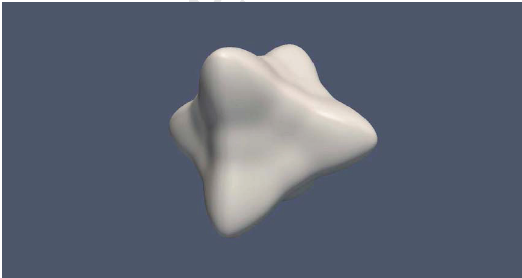
Figure 10: Dendrite image: Le = 40, \theta = -0.525, t = 102, dx = 0.78 . This simulation took 12 hours on a 12 core machine.
