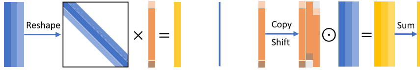
Fig. 3. Two approaches to evaluate the multiplication of a band matrix (stored with vectors) with a vector. The left figure corresponds to the case in Algorithm 2 and the right one is used in the implementation. The symbol \odot stands for element-wise multiplication.
