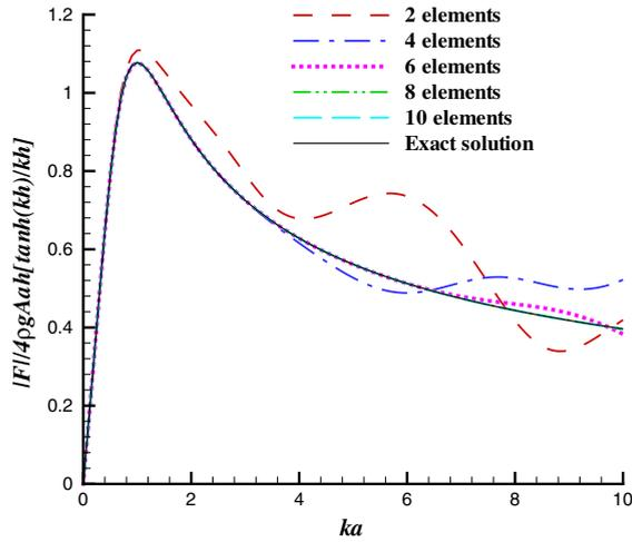
Fig. 6. The relationship between  $ka$  and the required elements number for wave forces on a circular cylinder.
