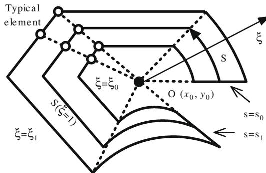
Fig. 2. The coordinate definition of SBFEM.
