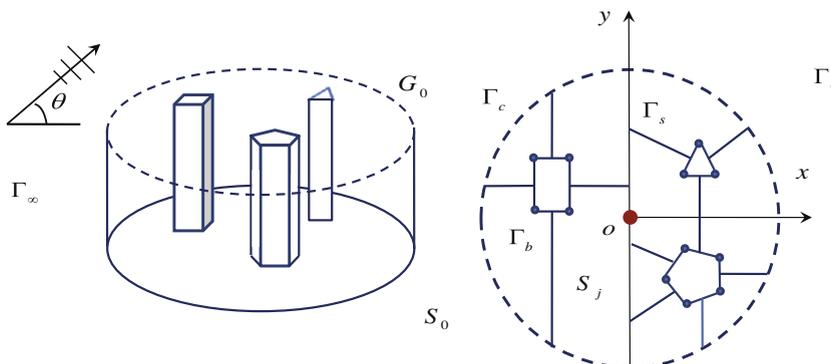
Fig. 1. A sketch of the water wave diffraction by multiple bodies.
