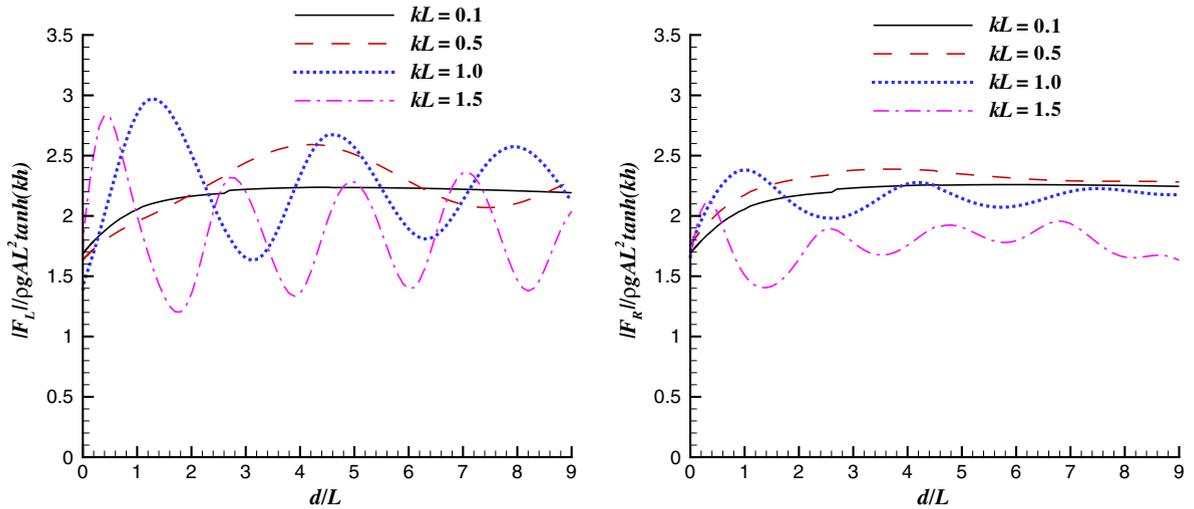
Fig. 16. Variation of nondimensional wave forces  $|F_x|/\rho g A L^2 \tanh(kh)$  on the twin cylinders vs. distance  $d/L$ .
