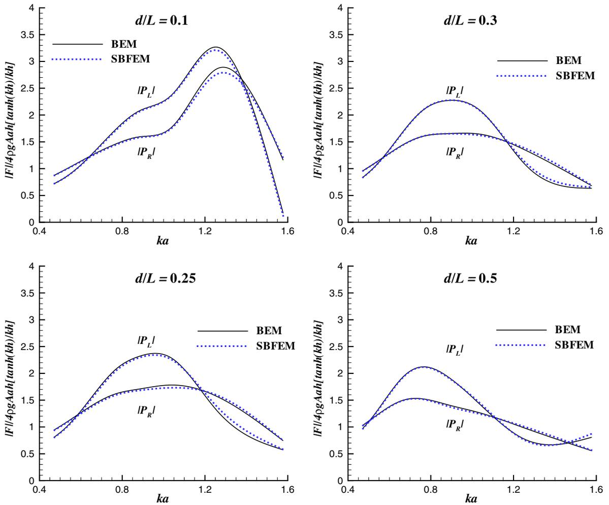
Fig. 14. Comparison of the nondimensional wave forces  $|F_x|/4\rho g A a h [\tanh(kh)/kh]$  on the twin cylinders vs.  $ka$ .
