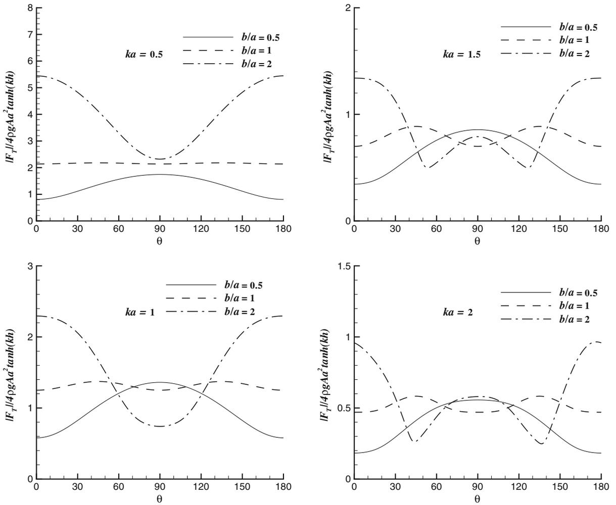
Fig. 10. Variation of nondimensional wave forces on the rectangular cylinder vs. incident wave angle  $\theta$ .
