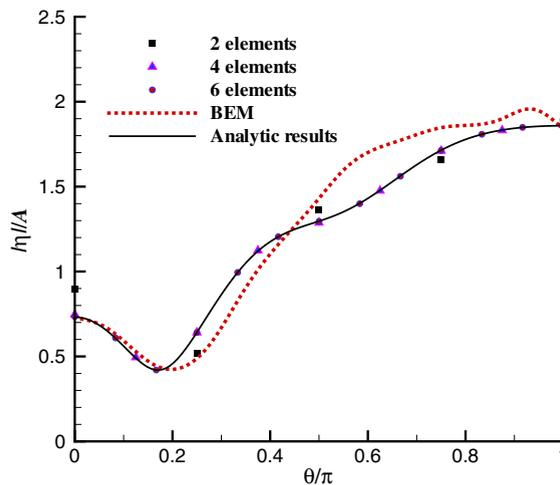
Fig. 5. Wave run-ups on a circular cylinder ( $ka = 2.0$ ).
