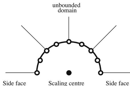
Fig. 3. Scaled boundary finite-element mesh for a circular cylinder.
