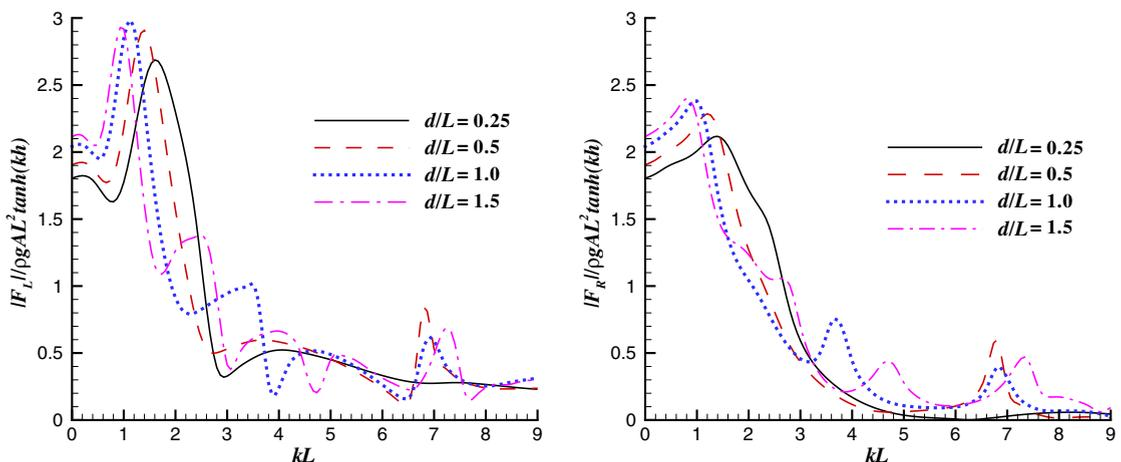
Fig. 17. Variation of nondimensional wave forces  $|F_x|/\rho g A L^2 \tanh(kh)$  on the twin cylinders vs. side length  $kL$  at incident wave angle  $\theta = 0$ .
