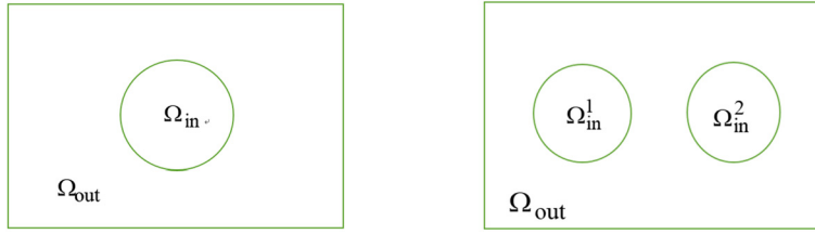
Fig. 2.1. The division of \Omega into atomic spheres \Omega_{\text{in}} and an interstitial region \Omega_{\text{out}} .
