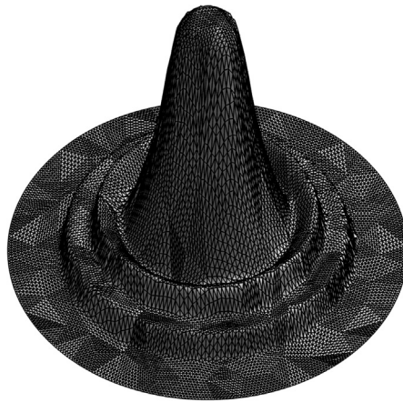
Fig. 22. Cross section of numerical solution of \rho in xy plane of 3-D explosion test with third-order WLS-ENO at t = 0.1 .
