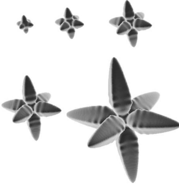
**FIG. 8.** Snapshots of a three-dimensional dendrite at  $\Delta = 0.1$  after 60,000, 120,000, 200,000, 300,000, and 650,000 timesteps (from top left). The computational parameters are given in the text and differ from those of Table I used in two-dimensional simulations.
