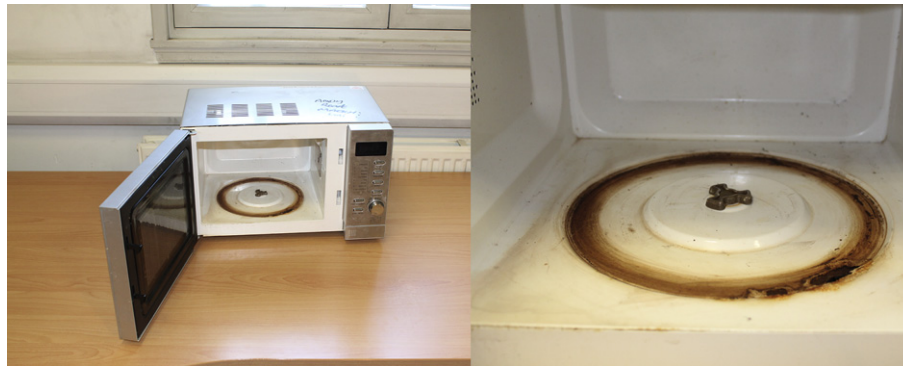
Fig. 6. Microwave oven with rusted internal cavity. Note: Fig. 6 shows cavity rust caused by the turntable wheels wearing down and lifting the floor surface.
