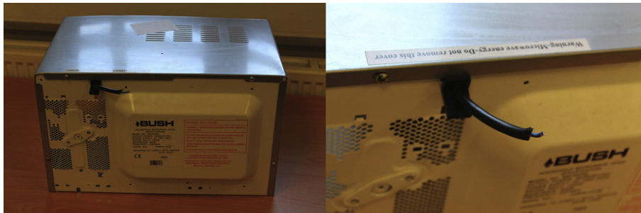
Fig. 8. Microwave with fixed cable (broken).
