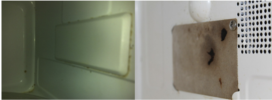
Fig. 7. Plastic and mica wave-guide cover. Note: Fig. 7 shows on the left an intact plastic type wave-guide cover, on the right a broken mica type wave-guide cover.
