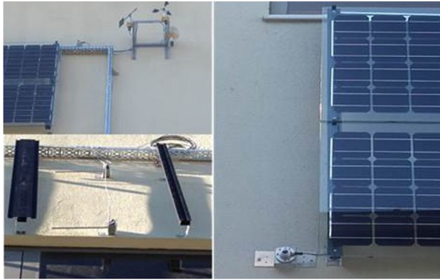
Fig. 6. Photos of the measuring devices including weather station and vertical pyranometer.
