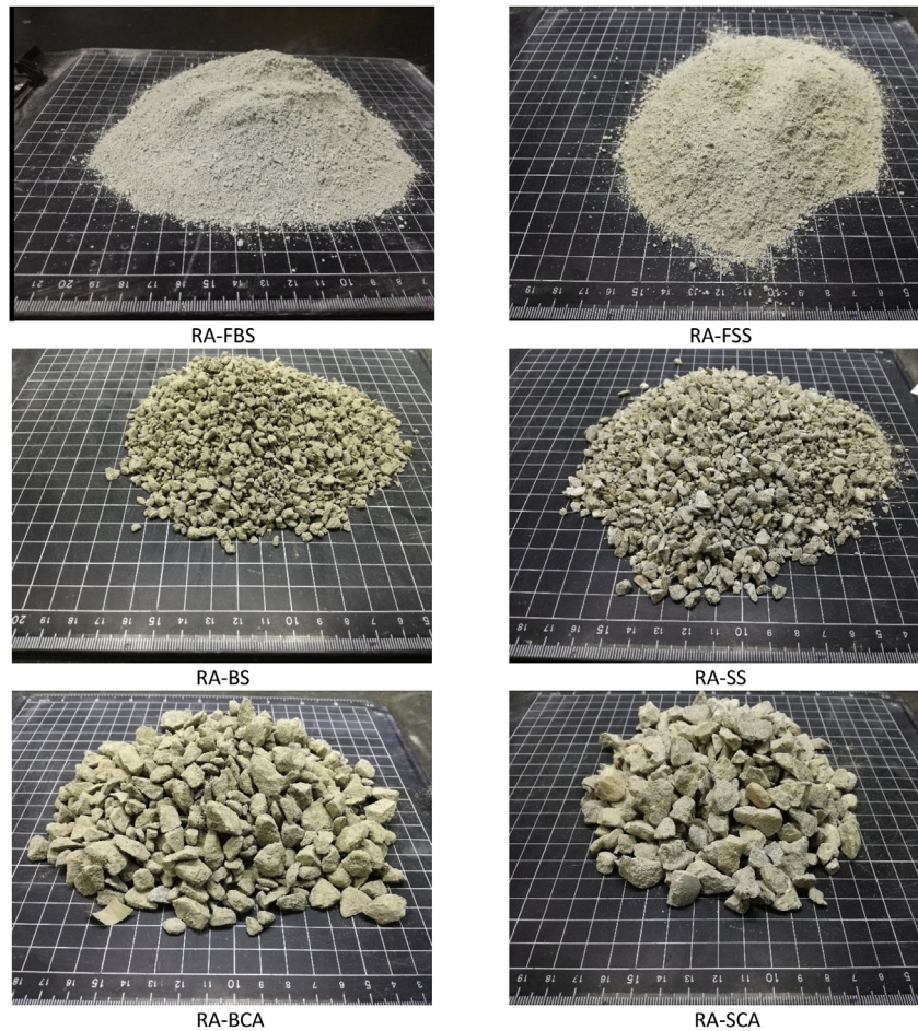
Fig. 2. RA produced using ballast and sleepers.
