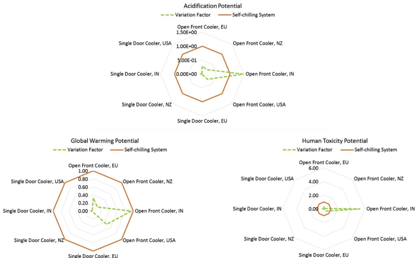
Fig. 6. Comparison of the self-chilling beverage can system with the base case and a conventional beverage aluminium can in Europe, USA, Indonesia and New Zealand.
