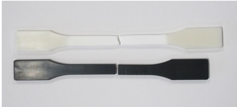
Fig. 1. Elongation to break evaluation-virgin ABS at top, 100% rABS below.
