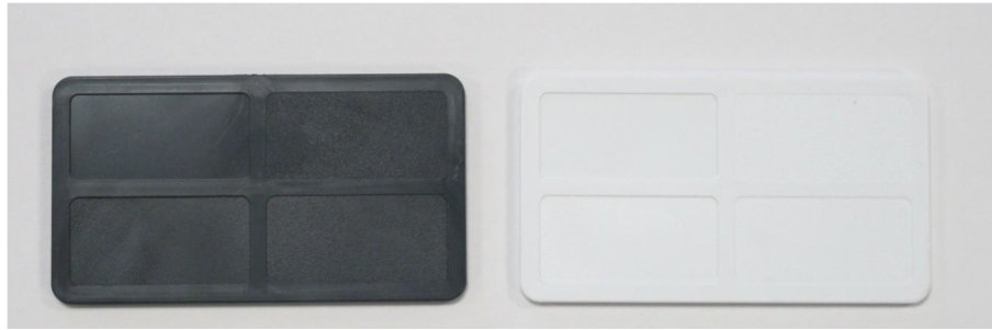
Fig. 4. Attempts to colour rABS compared to virgin ABS – rABS is on the left and virgin ABS is on the right.
