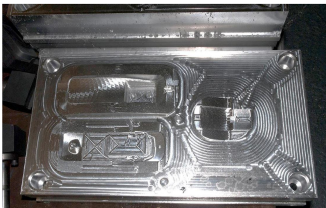
Fig. 14. Injection moulding tool.
