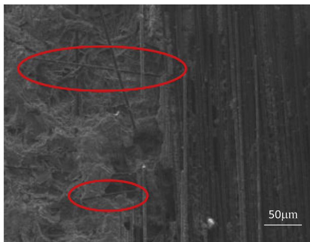
Fig. 11. Carbon fibers linked to multifilament yarns of a textile layer.
