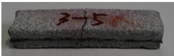
Fig. 8. Failure mode of the C-FRCM plates.
