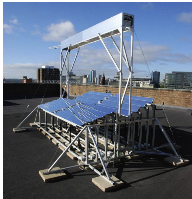
Fig. 14. The ELFR prototype, constructed on the roof at Aston University, UK.
