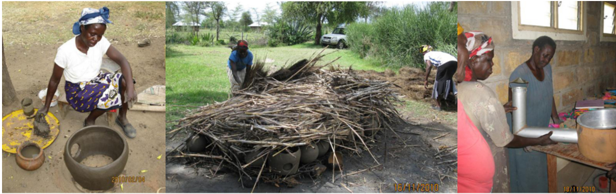
Fig. 2. Examples from the joint production and business chain for making and installing improved flue-piped stoves. The potter makes the co-designed stove from locally collected clay and prepares the firing using dry grass and maize stover. The facilitator demonstrates a flue-piped stove for a smoke-free kitchen in a nearby community. In late 2012, more than 200 households in nine communities had purchased a stove. LUCSUS illustrates the full process in a film: http://vimeo.com/9371888
