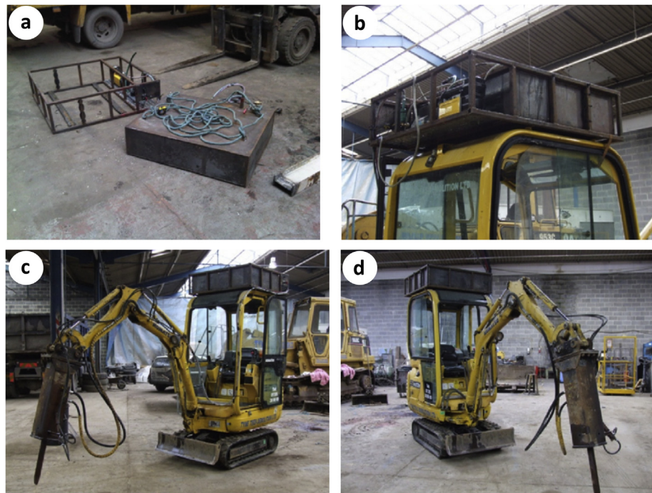
Fig. 7. The prototype system fitted into a mini excavator.
