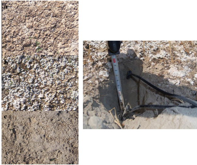
Fig. 1. Picture of the different types of surfaces and the moisture probes inserted in the soil: (a) cyanobacterial BSC; (b) lichen BSC; (c) BSC-scalped soil (6 months after BSC removal); and (d) installation of the moisture probes in the soil, at 0.03 and 0.10 m soil depths.
