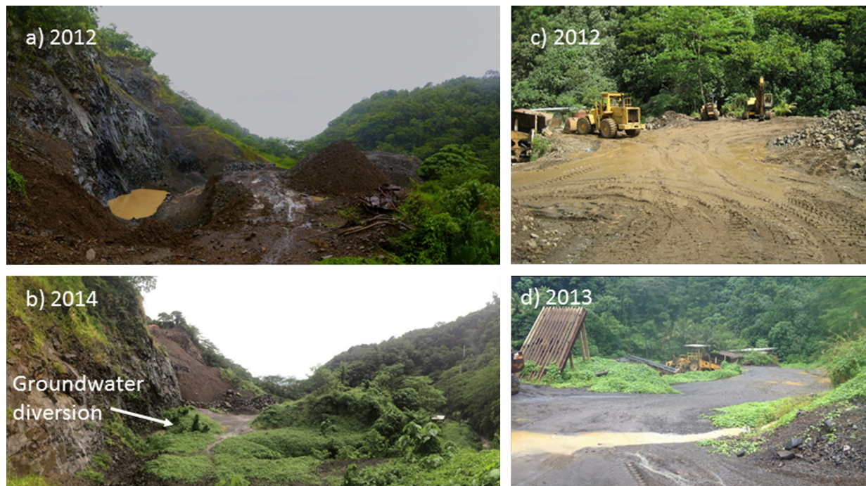
Fig. 2. Photos of the aggregate quarry in Faga'alu in 2012, 2013, and 2014. Pictures a–b show vegetation overgrowth during the period of study from 2012 to 2014, and the location of the groundwater diversion that was installed in 2012. Pictures c–d show that haul roads were covered in gravel in 2013. Photos: Messina.
